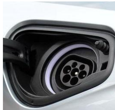
IEC 62196 Type2 Socket (install on Electric Vehicle)
