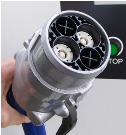
CHAdeMo Plug (install on charging station)
