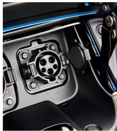
SAE J1772 Type 1 Socket (install on Electric Vehicle)
