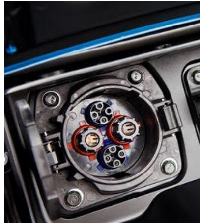
CHAdeMo Socket (install on Electric Vehicle)
